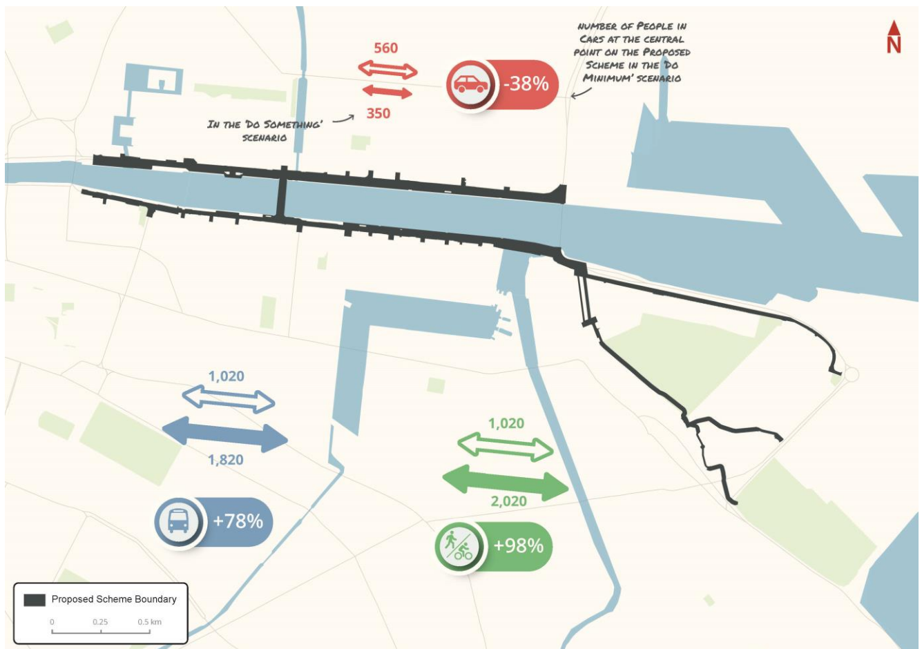
Diagram 6.6: People Movement by Mode travelling along the Proposed Scheme during 2043 PM Peak Hour
